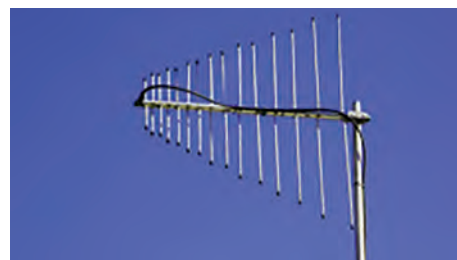
Antenna for the VHF and UHF bands.
