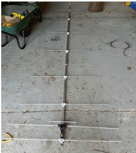
G4FAL's homebrew nine-element 2m band Yagi antenna.
