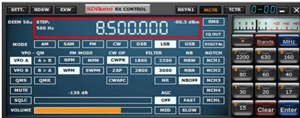
Figure 4. Main VFO setting in the RX Control console
