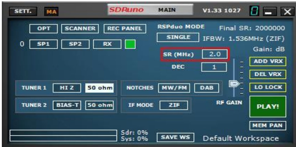
Figure 3. Bandwidth setting on SDRuno Main Console
