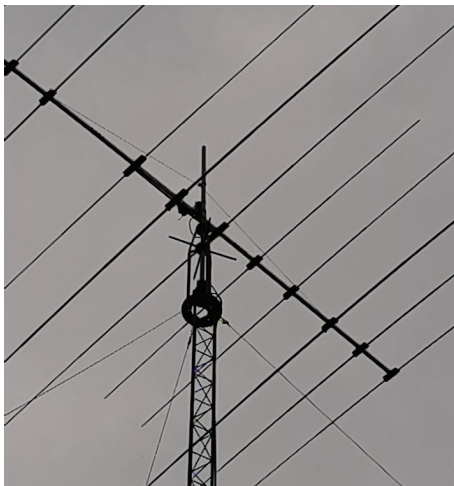
PHOTO 4: The G4FAL HF Yagi at 80ft (24.4m).
