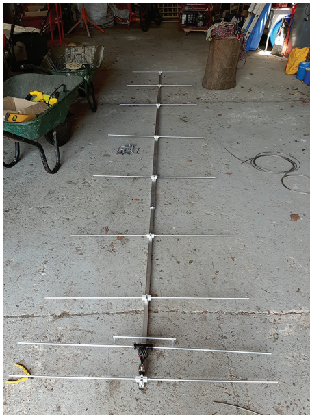
PHOTO 5: G4FAL's homebrew 9-element 2m Yagi.
