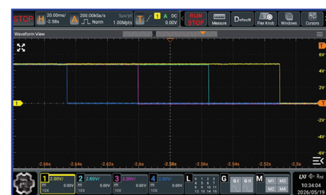
FIGURE 8: Oscilloscope capture of PTT turning off.
