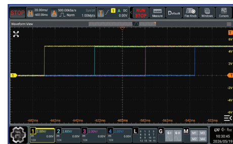
FIGURE 7: Oscilloscope capture of PTT turning on.
