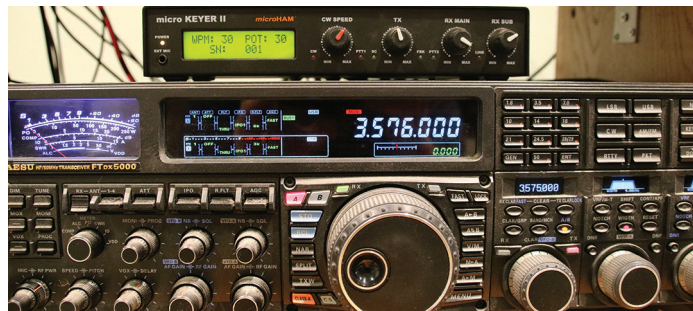
PHOTO 2: Microham MicroKeyer II interface used with Yaesu FTD5000.
