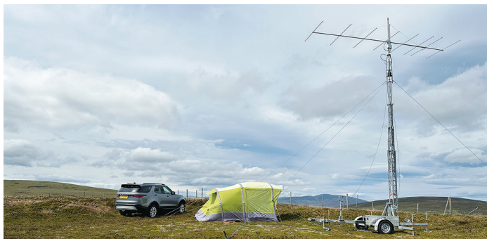
PHOTO 1: Alan, GM4ZUK's portable contest station with mobile tower ensures a competitive entry in many contests.
