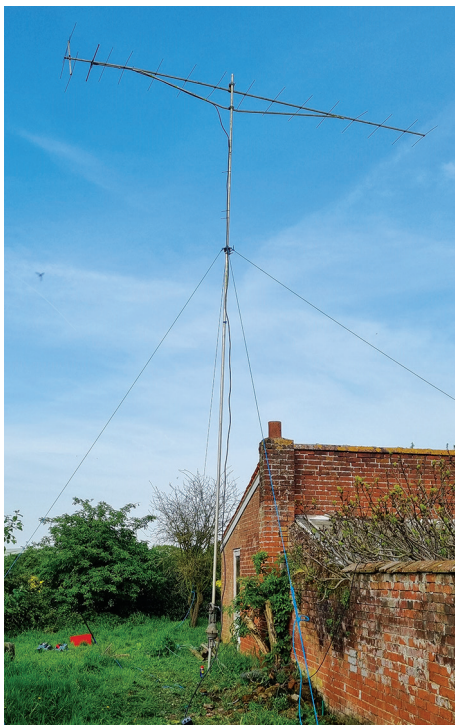
PHOTO 3: G4PIQ's simple 2m antenna – 17 elements on a 11m mast made from bits to hand.
