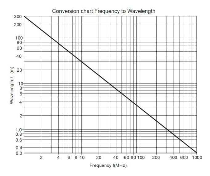
The velocity of radio waves is  $3\times10^8$  m/s or 300,000,000 m/s
