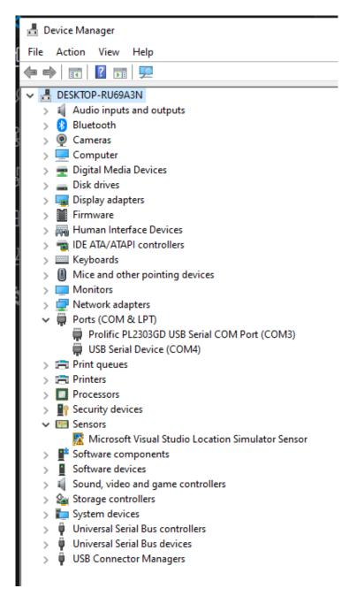
As you plug and unplug the USB cable to your Heltec Wireless Tracker board, look at the list of devices detected by "Device Manager". Under Ports (COM & LPT) you should observe a Windows "USB Serial (COMX)" device (where X is a number) appear as you plug in and unplug the USB cable. As shown in the Screenshot above, Windows reports the device as COM4 on my Windows 11 PC. On your Windows PC this number might be different so make note of it before moving on to the next stage
