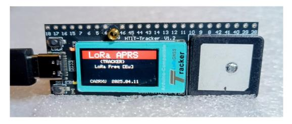
If all is well, it should display "LoRa APRS" on the 0.96" OLED, as shown in the image above.
