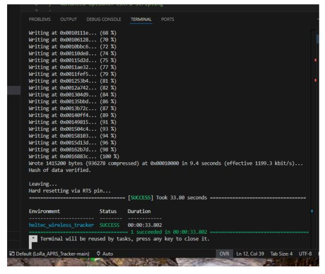
As soon as VSC has finished uploading firmware.bin and performed a hard reset, you should observer the Heltec Wireless Tracker board spring into life.
