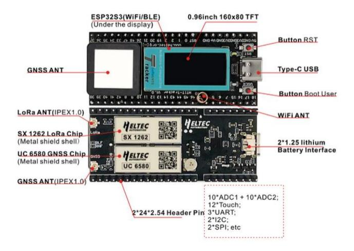
To upload the "firmware.bin" image (create by VSC) to the Heltec Wireless Tracker board, it is necessary to connect your Heltec Wireless Tracker board to your Windows PC via USB. You need a USB-C to USB-A lead, the same type use to charge Android mobile phones. Plug the USB-A end into a spare USB-A slot on your PC, and the USB-C end into the Heltec Wireless Tracker board. The first time you do this Windows will pop-up a message window about installing drivers for a "USB JTAG/Serial".
