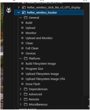
With the Heltec Wireless Tracker board still connected to your Windows PC (via USB), select "Upload Filesystem Image" and then observer the debug output in the TERMINAL window. You should observe VSC converting "tracker\_conf.json" to a format for uploading (a file called spiffs.bin) and then actually uploading it. If all goes well you should see "SUCCESS" displayed in green multiple times in the TERMINAL window, as shown below:
