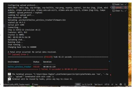
beeping noises as it detects the serial USB interface once again. With the ESP32-S3FN8 microprocessor now into bootloader mode, click on the white arrow (pointing right) on the bottom tool bar to perform the upload of firmware.bin once again.
